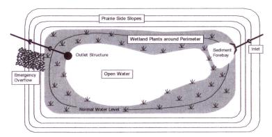
The detention pond's depth influences its water quality. Generally, detention ponds should be deep enough to maintain open water areas and limit sediment resuspension by current, wind, or waves. Typically, the average depth should be at least 4-5 feet and maximum depth at least 8 feet. If you want fish to survive through the winter, it is generally recommended that at least 25% of the pond be at least 10-12 feet deep.
