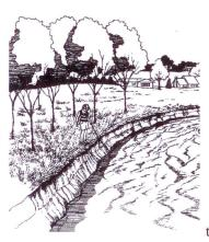
Pond shorelines often are designed too steep, making it difficult to establish stabilizing vegetation. Furthermore, detention pond shorelines typically have been planted with turfgrasses such as Kentucky bluegrass. Turfgrasses are too shallow-rooted to hold shoreline soils against the action of waves. They also cannot survive
